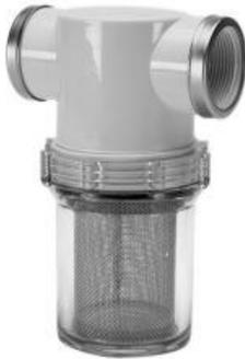
Mount the sea strainer with the provided 3/4" NPT nylon nipple directly to the intake of the 20 micron pre-filter housing. If an optional boost pump is required (refer to "Available Options and Accessories"), mount the sea strainer in a serviceable location in between the sea-cock of your choice and the boost pump.
